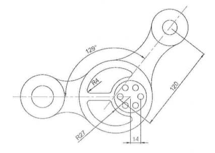
Draw the above figure using AutoCAD Commands
