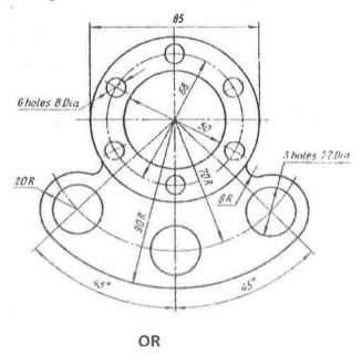
Q.1(B) Draw the below figure using Auto CAD commands
