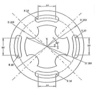
Draw the above figure using AutoCAD Commands
